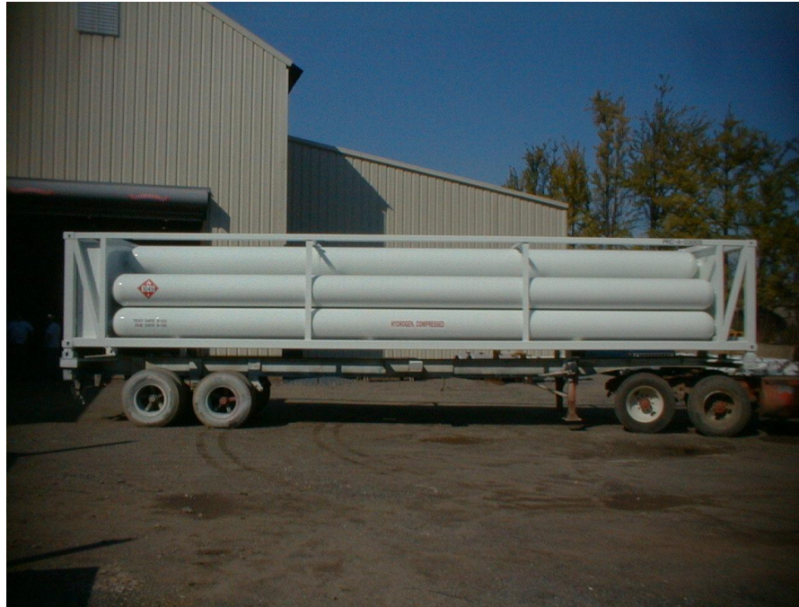
10 tube 40' ABS Skid (3T 36' tubes); 2400/2640 PSI.
