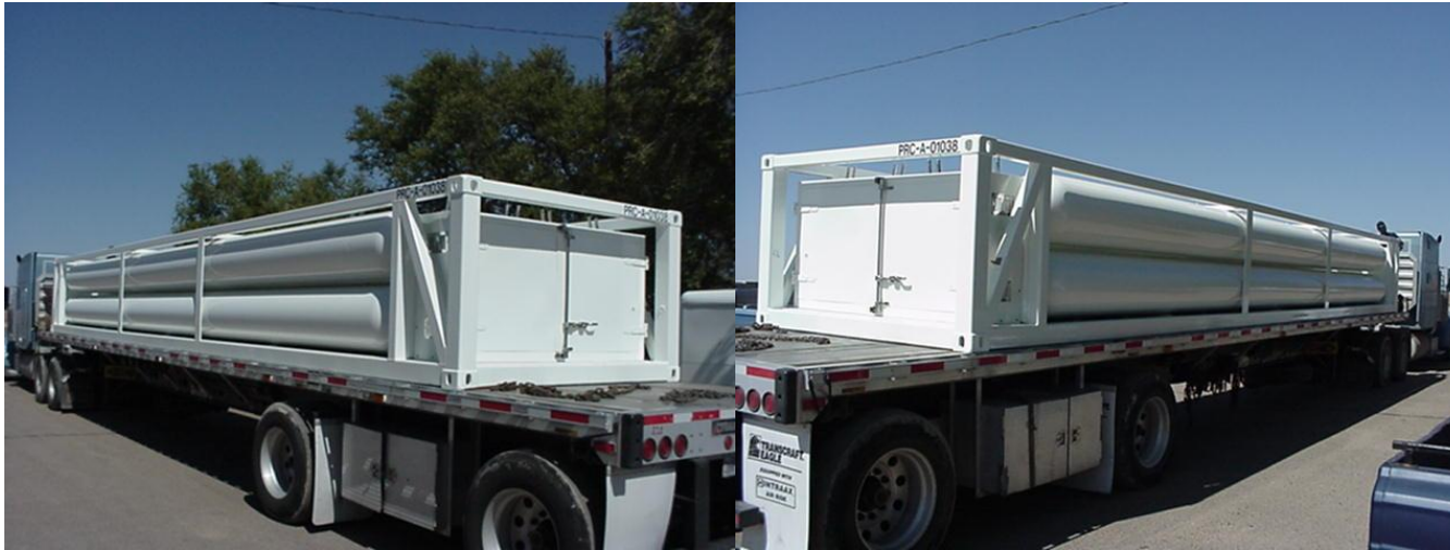
8 tube 40' ABS Skid (3T 36' tubes); 2400/2640 PSI.
