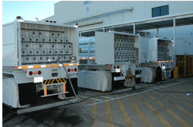
**MOBILE<sup>AE</sup> is an economical tool for cylinder recertification. Tubes are tested on the trailer using a lower test pressure than hydrotesting.**
