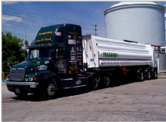
13 Tube Tri Axle Jumbo Hydrogen Trailer.
